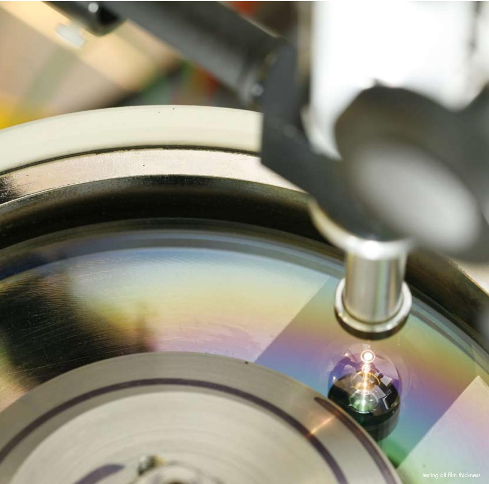
Testing oil film thickness
